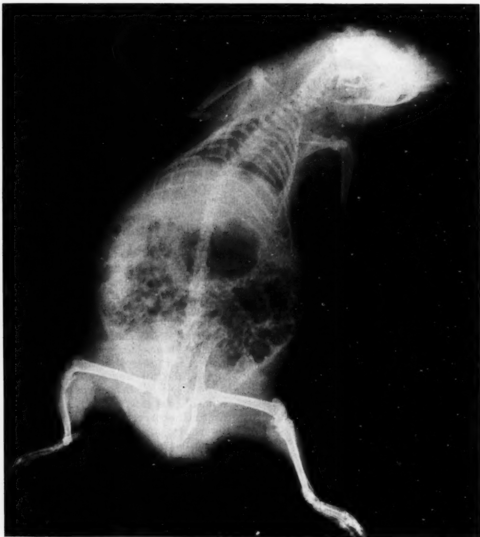
Fig. I-15 Radiograph of guinea pig made with a 1.96-curie I^{125} source. Time, 1.5 hr; distance, 10 in.; film, Du Pont Cronar with no intensifying screen.
